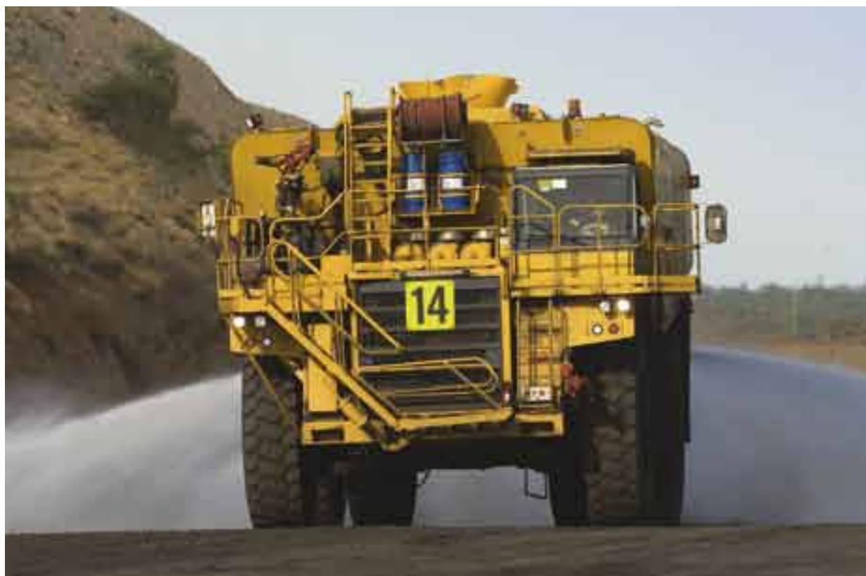
Water truck spraying to suppress dust on mine roads at Curragh.
