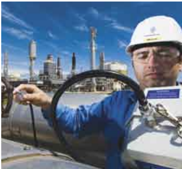
Process Operator Mark McCafferty performing a gas detection test at the inlet manifold.
