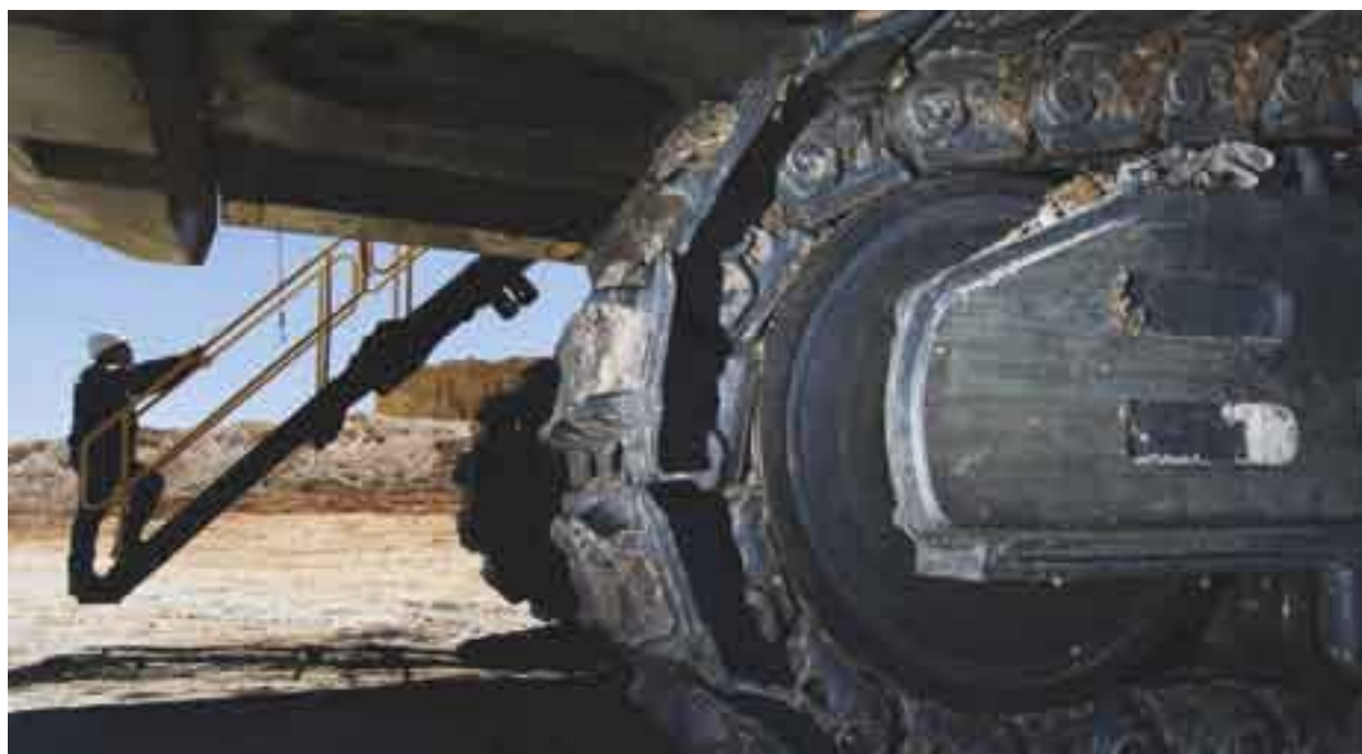
Access and egress to mobile equipment, a feature of safety training.
