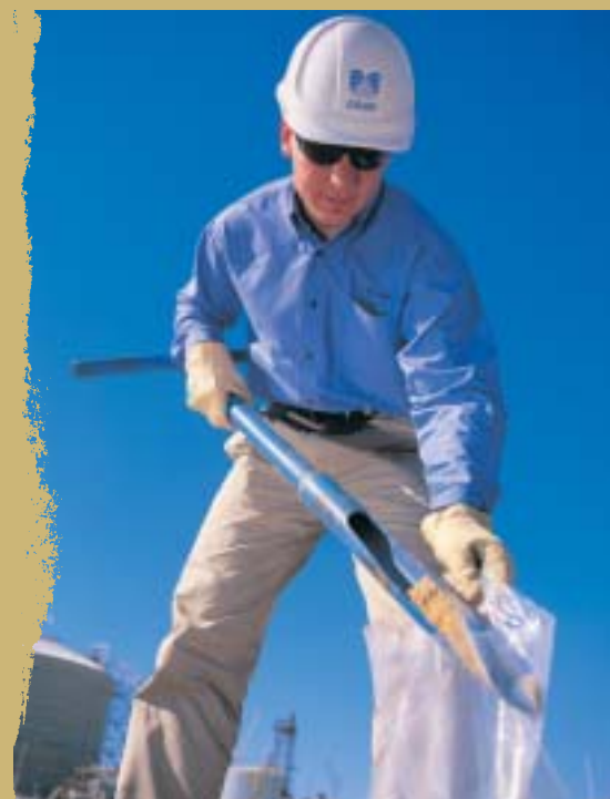
Kane Bennett taking soil samples at Kwinana as part of the preliminary site investigations required by Western Australia's contaminated sites legislation.
