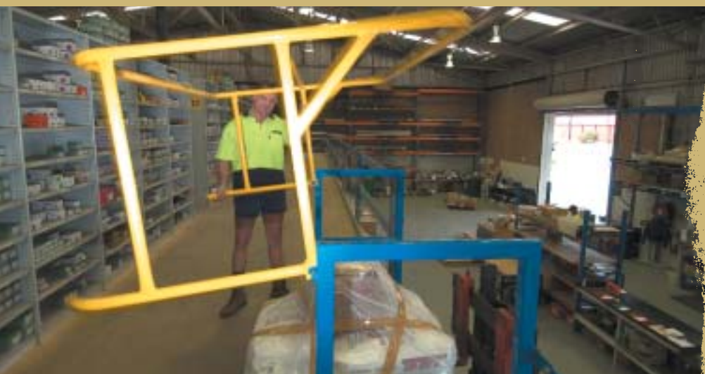
Operating a safety swing gate on a mezzanine level in the Mullings Fasteners distribution centre at Kewdale.
