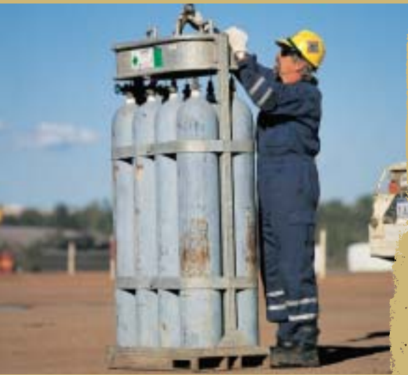
Dennis Ellis-Smith attaching new caged crates, specially designed to lift multiple gas cylinders, to a crane.
