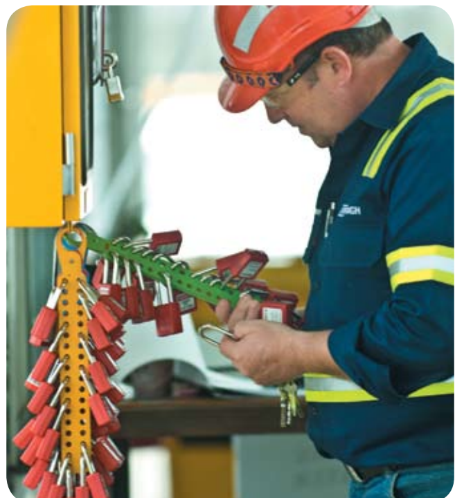
Curragh Safety Advisor David Banford locks onto the multi-lock out system for dragline 302 shutdown as part of the new isolation procedure.
